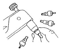
3. Squeeze tool to secure Rivet Nut.
