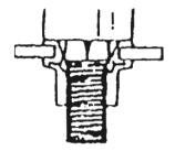
2. Thread Rivet Nut onto Nosepiece and insert it through hole in workpiece.
