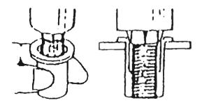
4. Unthread and remove tool from Rivet Nut.
