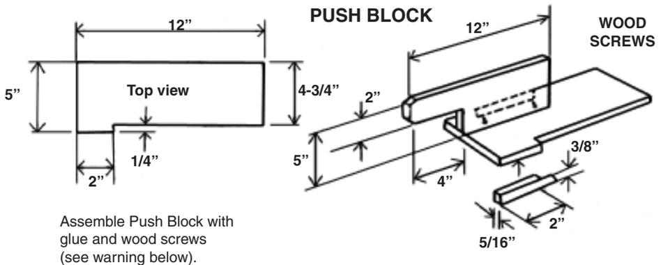
**WARNING!** When using wood screws, locate them so they will not accidentally come in contact with the saw blade.
