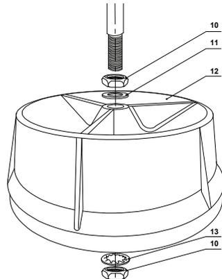
3. Use Lock Washer (13) and Nut (10) from underneath to secure the Shaft.
