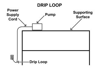
The "drip loop" is that part of the cord below the level of the receptacle, or the connector if an extension cord is used, to prevent water traveling along the cord and coming in contact with the receptacle.
