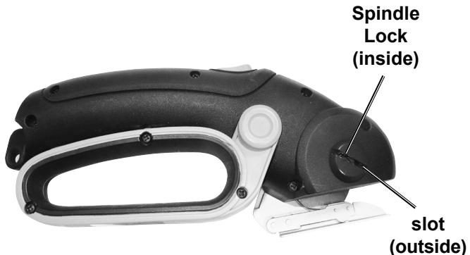
2. While holding Spindle Lock with screwdriver, Remove Blade Screw with another screwdriver.
