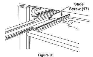
b. Gently pry the Cabinet Slide outward in the location shown and raise the end of the Cabinet Slide to disengage it.
