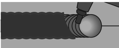
PARTIALLY CHIPPED AWAY TO SHOW WELD
