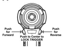
NOTICE: Do not change direction of rotation while Anvil is rotating. Wait until Anvil has come to a complete stop before changing direction.
