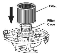
b. Secure Filter with Locking Cap.
