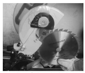
Figure G: Removing Blade
