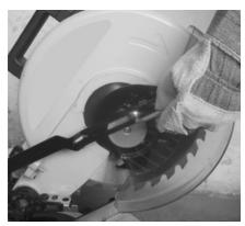
Figure D: Removing Safety Screw
