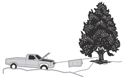
Figure A: Whiplash Dampening Blanket or Winch Damper
