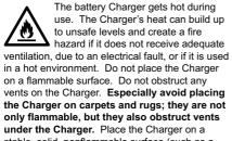
stable, solid, nonflammable surface (such as a stable metal workbench or concrete floor) at least 1 foot away from all flammable objects, such as drapes or walls. Keep a fire extinguisher and a smoke detector in the area. Frequently monitor the Charger and Battery Pack while charging.
