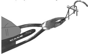
2. Lock the jaws in place by sliding the locking sleeve into the notch on the lever.
