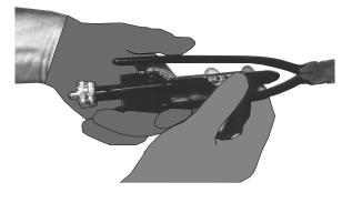
3. Grip the knob and pull straight back, allowing the tool and the wire to twist.
