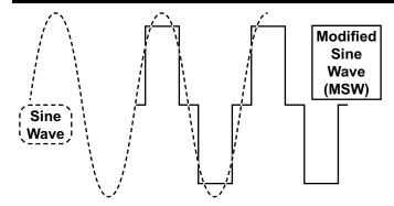
This Inverter's output is a Modified Sine Wave.
