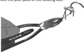
2. Lock the jaws in place by sliding the locking sleeve into the notch on the lever.
