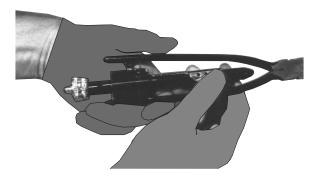
Grip the knob and pull straight back, allowing the tool and the wire to twist.
