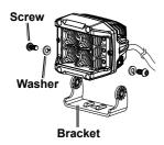
Point Light upward and place Bolt (3) through hole in the Bracket. See below.
