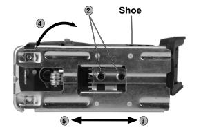
Use the Orbital Action Switch to set one of the following cutting modes:
