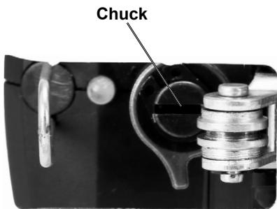
2. Install Blade with teeth pointing toward front of Saw.
