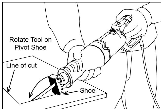
6. When the cut is complete, turn off the tool. Allow the tool to stop completely before removing it from the cut.
