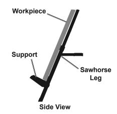
b. Place Workpiece on Supports.
