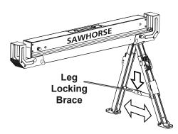
4. Above the location labeled "Close 1st" press the release button and pull Legs all the way down.
