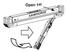
3. Separate Legs and push the Leg Locking Brace down flat.
