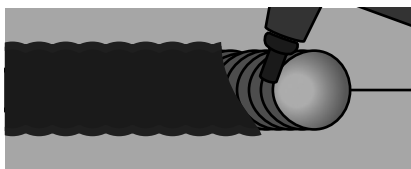
PARTIALLY CHIPPED AWAY TO SHOW WELD
