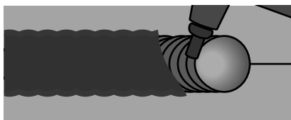
PARTIALLY CHIPPED AWAY TO SHOW WELD
