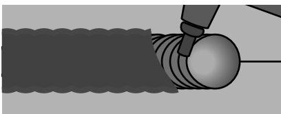
PARTIALLY CHIPPED AWAY TO SHOW WELD
