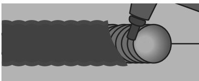
PARTIALLY CHIPPED AWAY TO SHOW WELD
