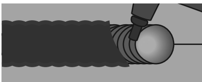
PARTIALLY CHIPPED AWAY TO SHOW WELD
