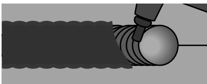
PARTIALLY CHIPPED AWAY TO SHOW WELD
