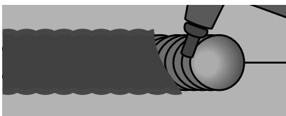
PARTIALLY CHIPPED AWAY TO SHOW WELD
