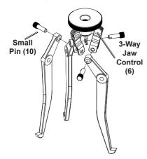
Connect Three Jaw Yoke (8) to three Jaws. Insert three Large Pins (11) through either inner or outer holes. Use same hole on each side.
