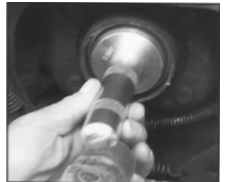
Installing new Bearing
