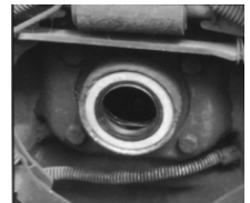
New Seal installed
