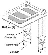
Attach the Swivel Casters (5) to the Platform (4) near the Handle Bracket (3) using Washers (7) and Bolts (8).
