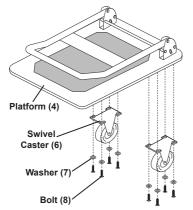
Attach the Swivel Casters (6) to the Platform (4) near the Handle Bracket (3) using Washers (7) and Bolts (8).
