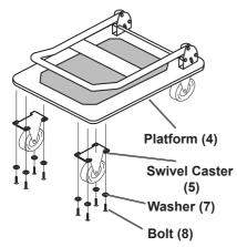
1. Attach the Swivel Casters (5) to the Platform (4) near the Handle Bracket (3) using Washers (7) and Bolts (8).
