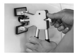
Slowly squeeze the Lever Puller's handles until there is a pop and the dent is raised. Stop when dent returns to normal surface level. Turn knob, if necessary, to increase pull.
