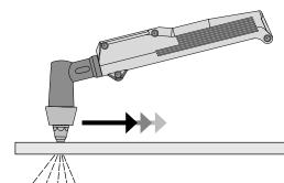
8. Slowly move the Torch along the cutting line with the Cutting Tip trailing.
