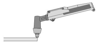
12. Release the Trigger. The air will continue to come out of the Torch for a few seconds once the Trigger is released to cool off the Torch components.
