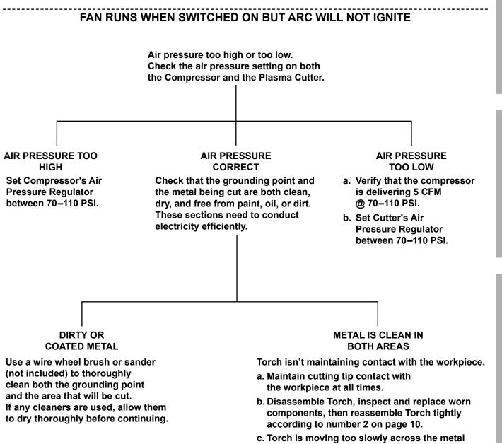
c. Torch is moving too slowly across the metal and cutting the material from underneath, breaking contact. Move Torch more quickly. SAFET
