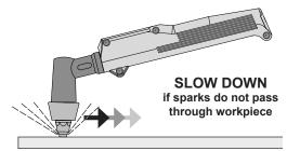
9. If sparks start shooting up from the workpiece instead of passing through, the Torch is being moved too quickly so the cut is not being made completely. Move the Torch along the workpiece more slowly to cut completely.
