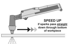
10. If sparks pass straight down through bottom of workpiece instead of at a slight angle, the Torch is being moved too slowly. This could cause the arc to extinguish. Move the Torch a little faster.
