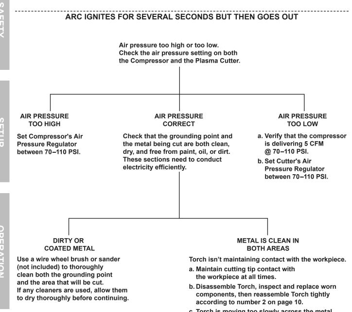
c. Torch is moving too slowly across the metal and cutting the material from underneath, breaking contact. Move Torch more quickly.
