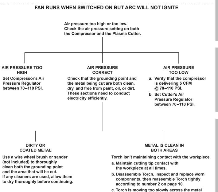
c. Torch is moving too slowly across the metal and cutting the material from underneath, breaking contact. Move Torch more quickly. SAFETY
