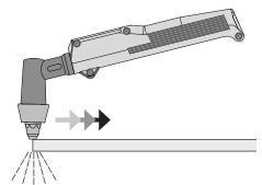
7. **Do not press Trigger until Torch is in position to start cutting.** Starting at the edge of the workpiece, press and hold the Trigger to strike the pilot arc. When the arc ignites, start slowly moving the Torch along the cut line.
