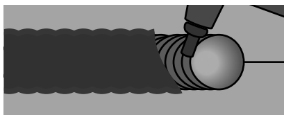
PARTIALLY CHIPPED AWAY TO SHOW WELD
