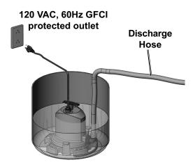
**Note:** The Pump must be in water at least 3/16" deep for it to operate properly.
