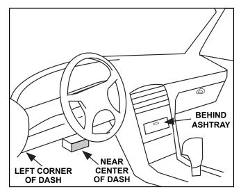
2. For most vehicles, use OBD2 Diagnostics/DoIP Cable to connect DLC and Scanner.
