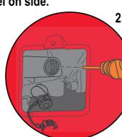
2. Pull the Oil Drain Hose out of the Generator. Remove the Oil Drain Cap. Drain Oil. Replace the Oil Drain
