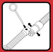
2. Install cutting head; use tool to remove
