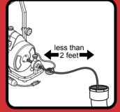
3. Position within 2 feet of drain opening
