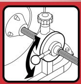
If the cable stops and tension builds, release foot switch, wait for tension to release, then pull cable back manually before proceeding.
