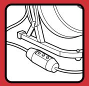
4. Plug in and press reset button on GFCI
