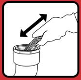
If the cable stops and tension builds, release foot switch, wait for tension to release, then pull cable back manually before proceeding.
