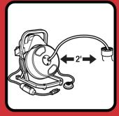
3. Position within 2 feet of drain opening
