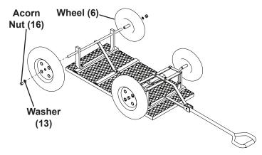
9. Test all bolts and nuts for tightness before turning the wagon over on its wheels. Roll the wagon to check for proper wheel operation. Periodically check tire inflation (maximum tire inflation is 30 PSI). Periodically lubricate wheel axles.
