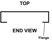
AWARNING! TO PREVENT SERIOUS INJURY: In the following assembly process, the flange pictured above must face down with the Tongue (2) edge fully contacting the tailgate. It is designed to keep the Ramps from moving once the weight of the load is riding on the Ramps.
