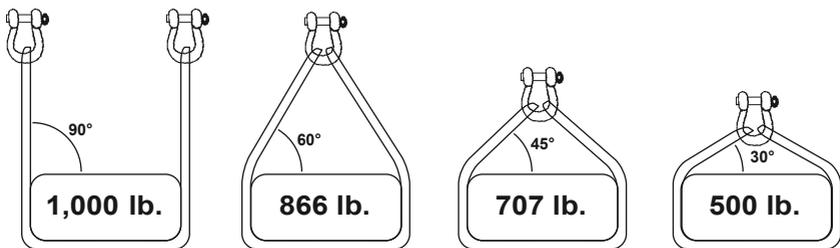
A sling capable of lifting 1,000 lb. in a 90° vertical basket hitch can only lift 866 lb. at a 60° angle, 707 lb. at a 45° angle, and 500 lb. at a 30° angle. Refer to other regulations, codes and standards for additional information and safe operating practices. See OSHA CFR 1910.184 Regulations, ANSI/ASME 830.9, and the Web Sling and Tie Down Association Standards.
