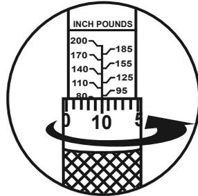
8. Tighten the Lock Knob by turning it clockwise until it stops.
