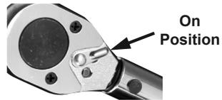
**Note:** Thread fastener with another tool until it is snug, then finish the operation with the Torque Wrench.
