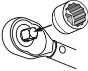
5. Loosen the Lock Knob by turning it counterclockwise until it stops.
