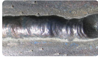
Weld Speed Too Slow
