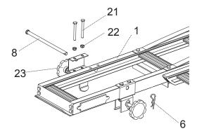
2. Install Lock Pins (8) and Adjustment Pin (16) into Platform. Secure with R-pins (6).
