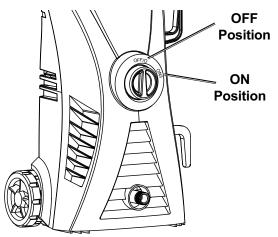
**<u>NOTICE</u>**: Pressure Washer will run **only** while Trigger is pressed. When trigger is released, Pump will turn off. **Do not leave idle for more than one minute without spraying.**
