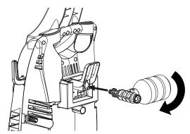
Store in a dry, frost-free room. Flush the unit with automotive antifreeze prior to long-term storage. Dispose of antifreeze according to local ordinances.
