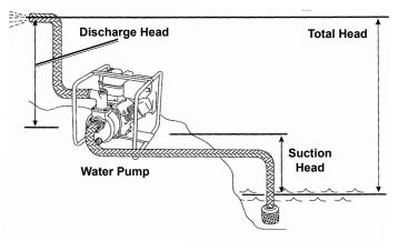
As the head (pumping height) increases, pump output decreases. A non-collapsible suction hose must be used. The length, type, and size of the suction and discharge hoses can significantly affect Pump output.
