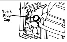
1. Disconnect spark plug cap from end of plug.
