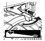
b. Turn the Engine Switch off.
