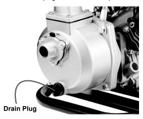
2. Tilt Pump forward to drain all remaining water from inside.
