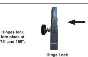
Pull Side Lock out, rotate to hole, then release into hole. Side lock must extend fully into hole.
